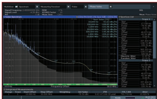
Fig. 4 An option enables measurement of the amplitude and phase noise of a signal.
